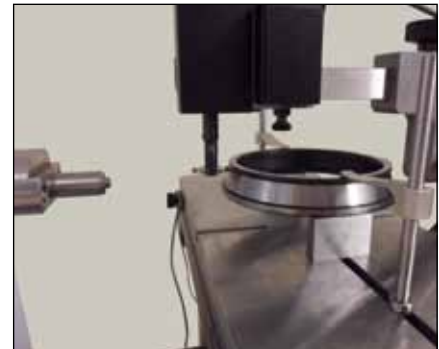
CNC controlled external taper ring measurement
