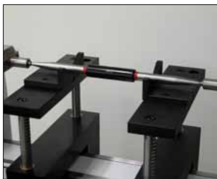
Calibration of gauge bars (TELEMA7/TELEMN7.2)
