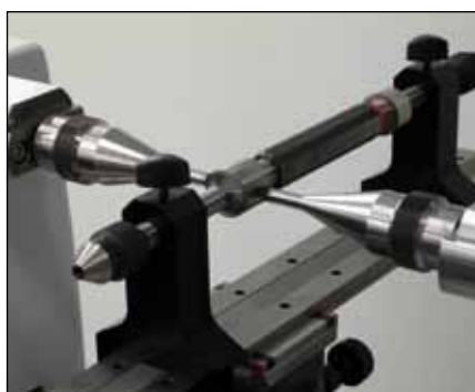
Calibration of plug gauges (TULM6/L05/TA-SU-315)
