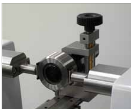
Calibration of thread plug gauges (3P/0.17-3.2/S6.5/TA-SU-315)
