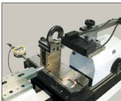
Checking of taper thread ring gauges (HPA-1/LABC80)
