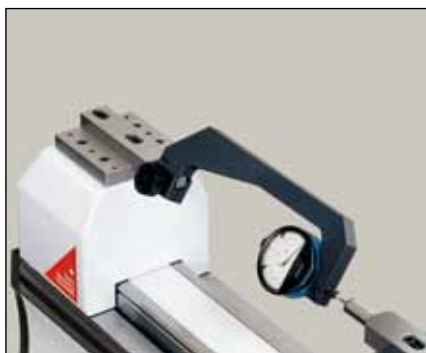
Checking of dial indicators (TULM5C)
