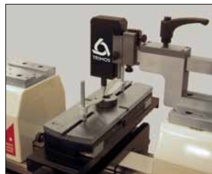
Calibration of small ring gauges (TA-SU-313/LABC-70/TA-SU-354)
