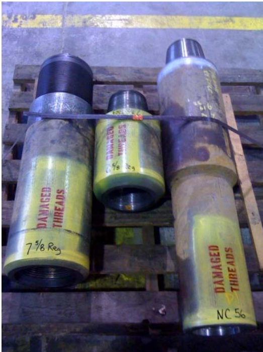
Figure 15: Damaged threads declared by Lewis Inspection Group.
