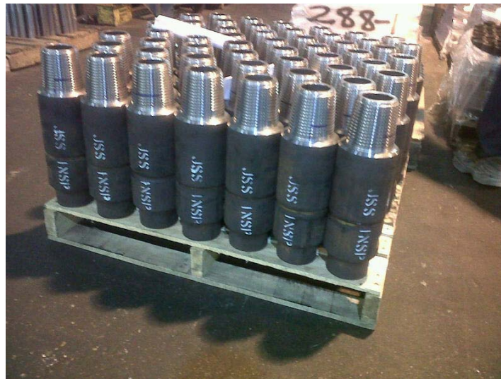
Figure 17: Tejas stamps each connection with “JSS INSP” which shows that they have not only been inspected to current API Specifications, but the precise pitch diameter has been measured and documented.
