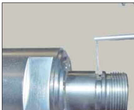
Checking at recessed measuring points (TA-MS-609)
