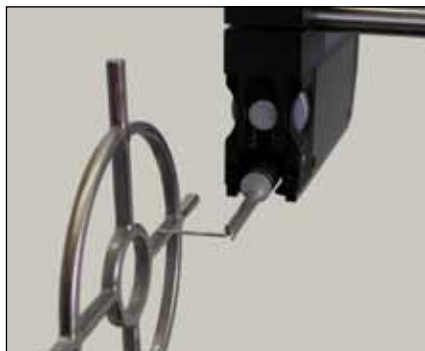
Transversal flank measurement (TA-MS-627)
