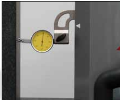
Squariness mechanically adjusted on all instruments
