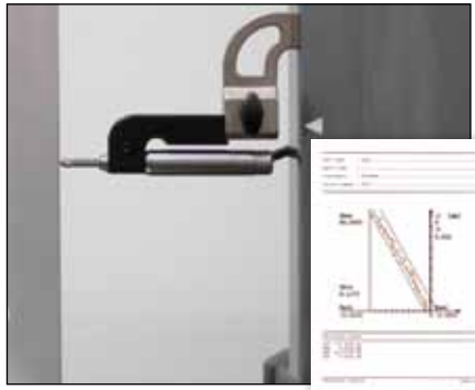
Checking of squariness using an additional electronic probe and colour print-out of the curve (TA-MS-101)
