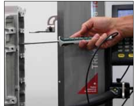
Measurement using temperature compensation system with optional external sensor (TA-EL-120)
